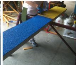
Ramps have contact zones Here the transition is made to yellow (note forms must be removed promptly)
